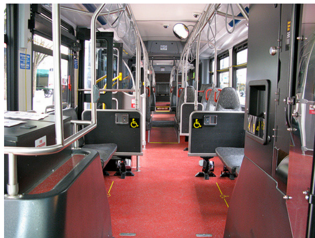
Wide aisles offer greater passenger comfort and ability to circulate within BRT vehicles
