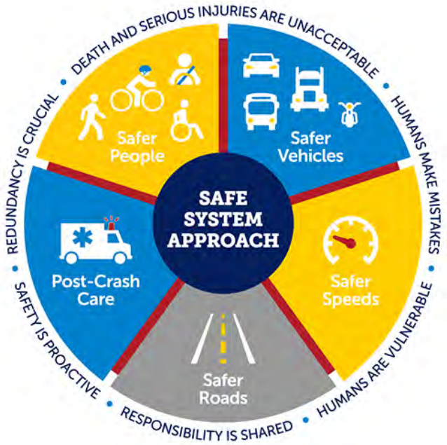
Figure 1.1 - Safe System Approach Source: US Department of Transportation, What is a Safe System Approach, 2025
