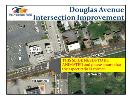
The Montgomery Road and Douglas Avenue intersection will be improved for operational efficiency and to provide additional capacity for future travel demand. The improvement includes restriping of the northbound approach to provide an exclusive right turn lane and a shared through-left turn lane. Pedestrian crosswalks will remain for the east, west, and north legs of the intersection.
